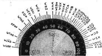
Grebe Dial All stations have equal spacing around the dial.
