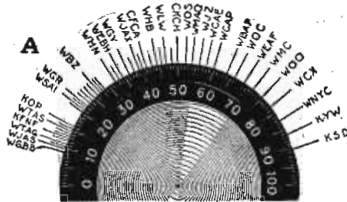
Grebe Dial All stations have equal spacing around the dial.
